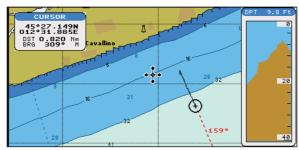
Fig. 3.1.2 - Example of Depth Graph 1/3 of the screen
