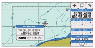
Fig. 4.1.1.1 - Waypoint placing
