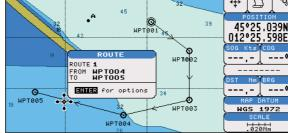
Fig. 4.1.1.7 - Placing Waypoint between two existing ones (I)
