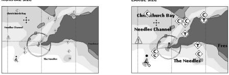
Fig. 3.5.1.5 - Example of Normal size (on the left side) and Large side (on the right side) settings
