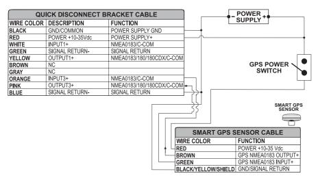
Fig. 7.4a - GPS Connection on Port 3 For PANORAMIC 8 HD FISH
