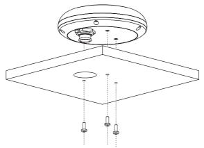
Fig.B.1b - Installing GPS Antenna (III)
