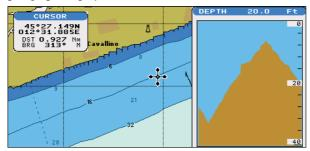
Fig. 3.1.2a - Example of Depth Graph 1/2 of the screen
