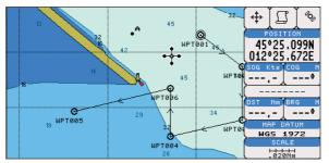
Fig. 4.1.1.7b - Placing Waypoint between two existing ones (III)
