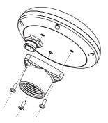
Fig.B.1 - Installing GPS Antenna (I)
