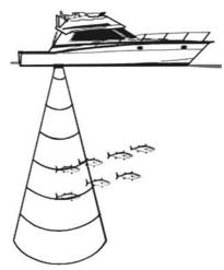
Fig. 6 - Fish Finder working principle
