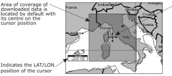
Cursor is locked to the gray area. Moving the cursor also moves the gray area allowing locating it over the area where the user wants to download the Meteo forecast.
