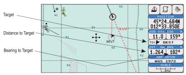
Fig. 3.4.1 - Navigation to a single destination
