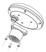
Fig.B.1 - Installing GPS Antenna (I)
